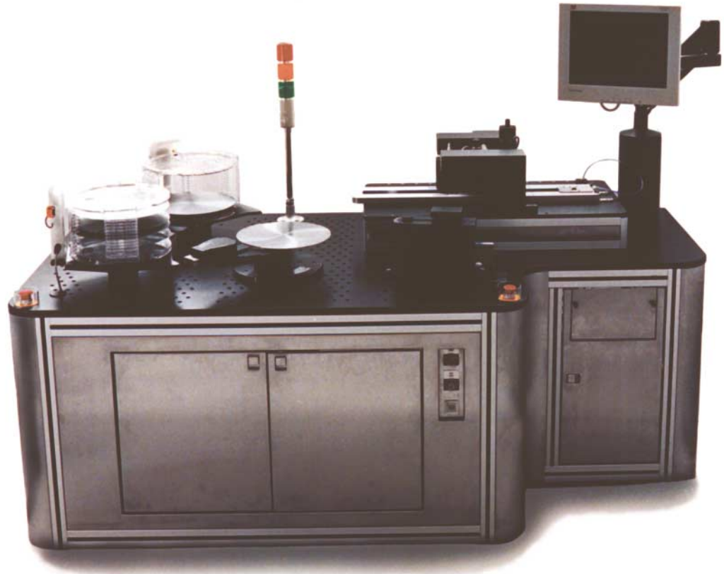
LEI RS300 (300 mm Robotic Sorting) shown with 2 cassettes (product may differ from photo)
